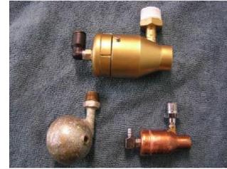
図 2 Gas-liquid two-phase flow whirling type microbubble generator
