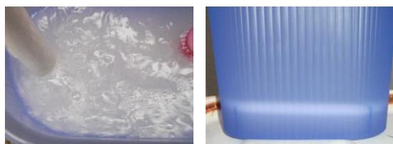
図 8 Emulsification of kerosene and water by use of the microbubble generator
