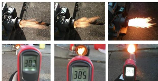
図 9 Temperature measurement results of flame by kerosene burner (Left pictures: kerosene (302 °C), Center pictures: kerosene + MB (385 °C), Right pictures: kerosene + water + MB (257 °C))
